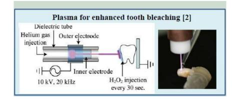
Figure 3: Schematic representation of a plasma apparatus for enhanced tooth bleaching [34].
